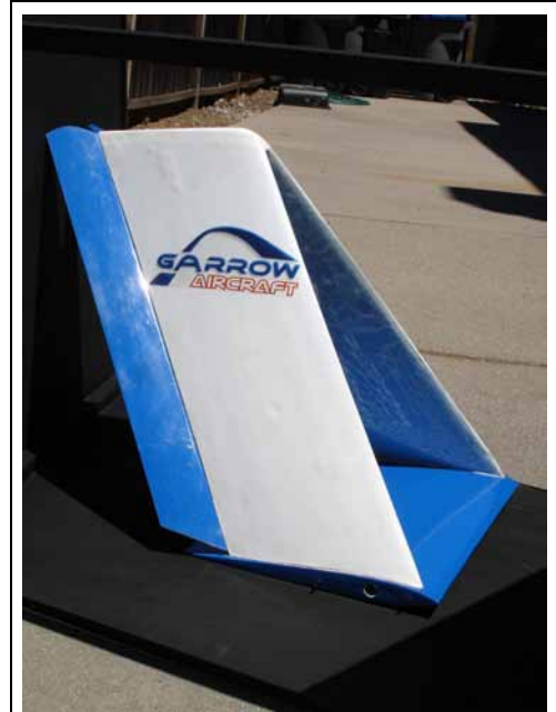
As a sneak preview, here is the V-tail assembly that was recently completed that only weighs 363 gr (9.7 oz).
